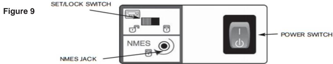
◆ **Note:** To prevent inadvertent loss of synchronism between the CPM and the chosen muscle stimulator, use only medical grade link cables with locking plugs. The NMES trigger jack will deactivate the muscle stimulator one second before the end of the Extension Pause Mode. Refer to the muscle stimulator instruction manual for proper set-up.
