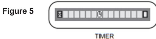
Time can be set in 10-minute increments up to 480 minutes (eight hours). Once the treatment session is over, a 480E device will run to the middle of the set range of motion and stop. The motion controller will display a flashing timer symbol. The operator must turn the device off and on again at the power switch to proceed (Section 2.1, Overview of Family of 480E Devices).
