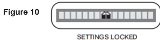
◆ **Note:** Attempting to change settings while the Lockout feature is engaged will result in the lock symbol appearing in the center display window.
